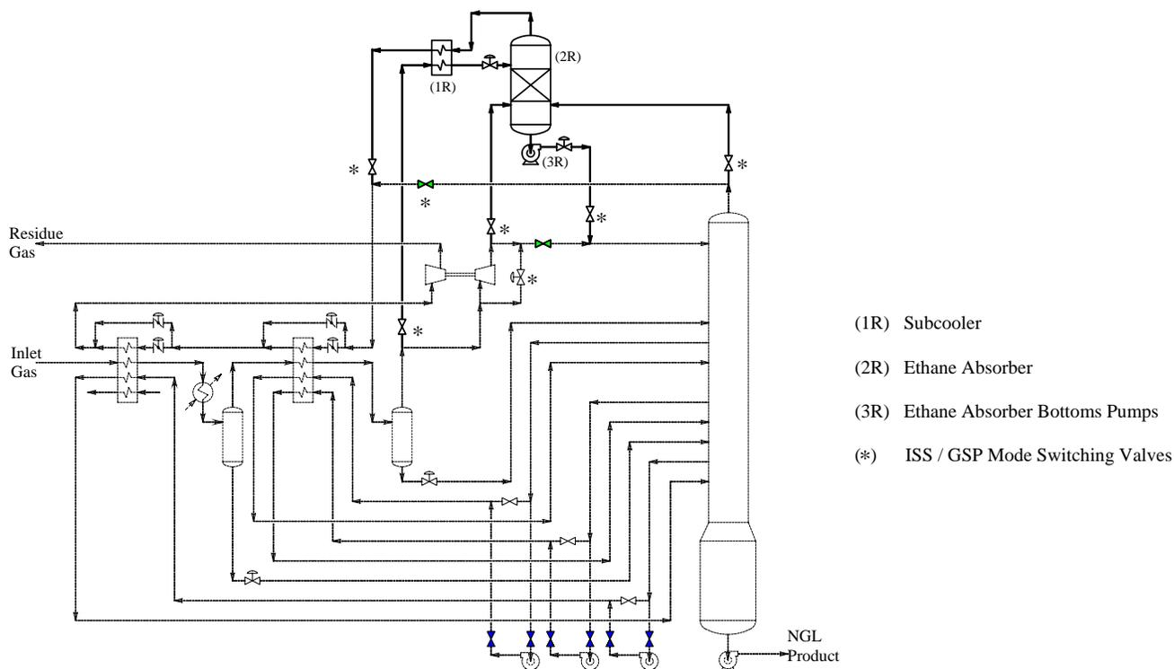
Figure 2 - GSP Retrofit Process Flow Schematic
