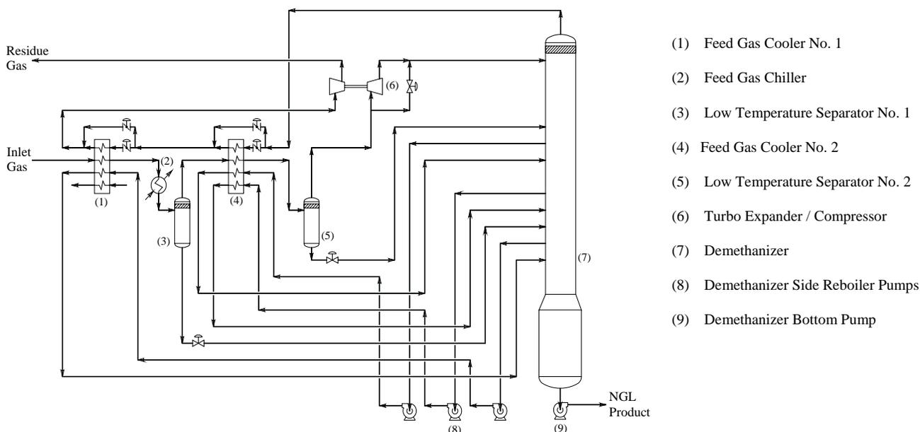
Figure 1 - LTSU Process Flow Schematic
