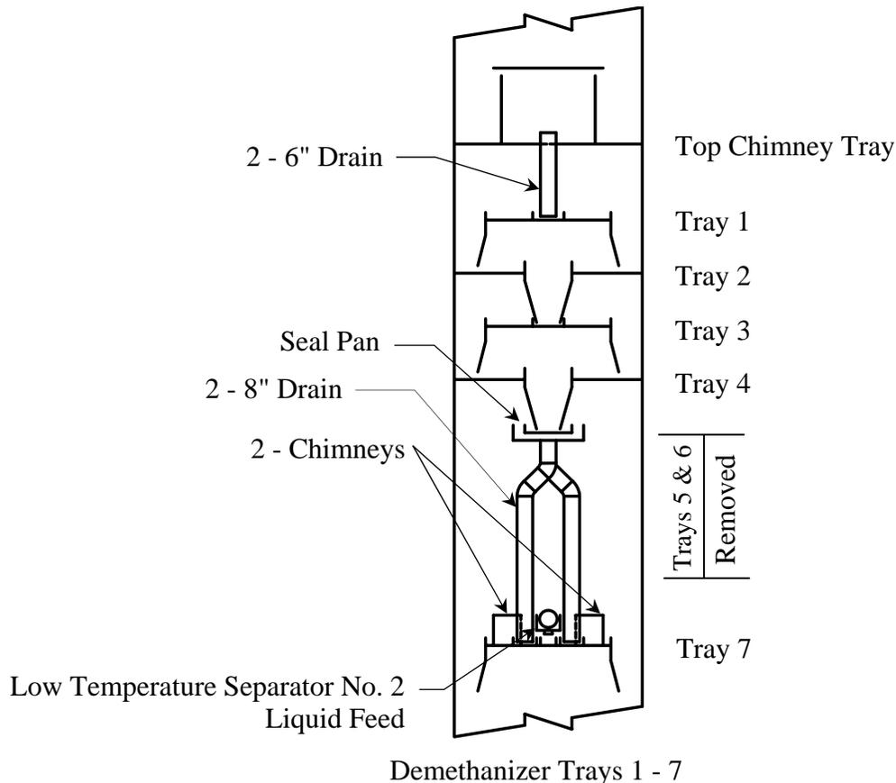
Figure 3 - Demethanizer Tray Configuration
