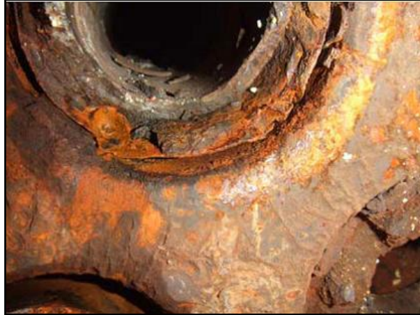
Figure 12. WHB Tubesheet Joint After One Year Service (From a non-Ortloff licensed unit, not one of the case history SRUs)
